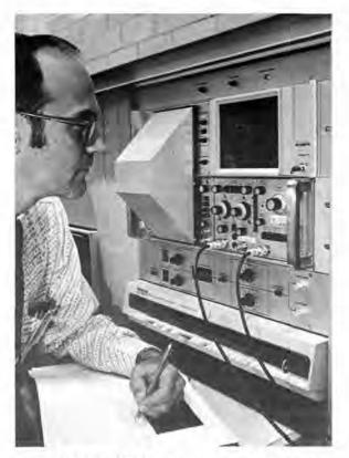
LABORATORY MODEL of the vidicon digitizer is checked by Thomas Evans (2342), a co-developer of the system. From top to bottom are oscilloscope, digitizer and computer.
